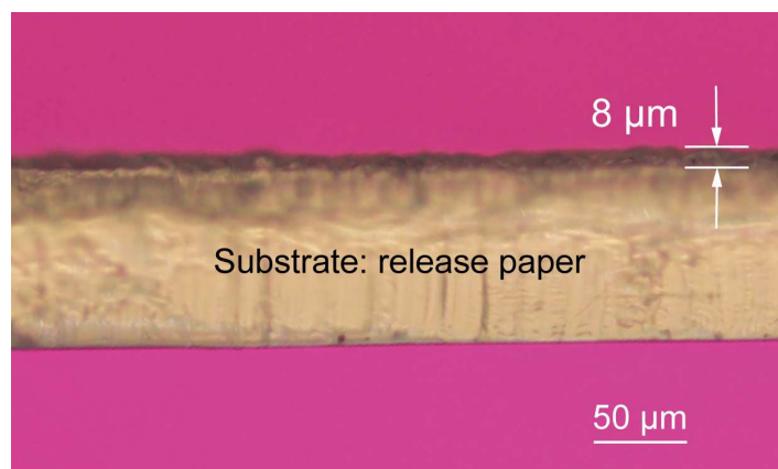
Supplementary Fig. 4. Thickness of pLCE ionic nanomesh. The thickness of the pLCE ionic nanomesh was measured to be \sim 8\ \mu\text{m} , as determined by optical microscopy.
