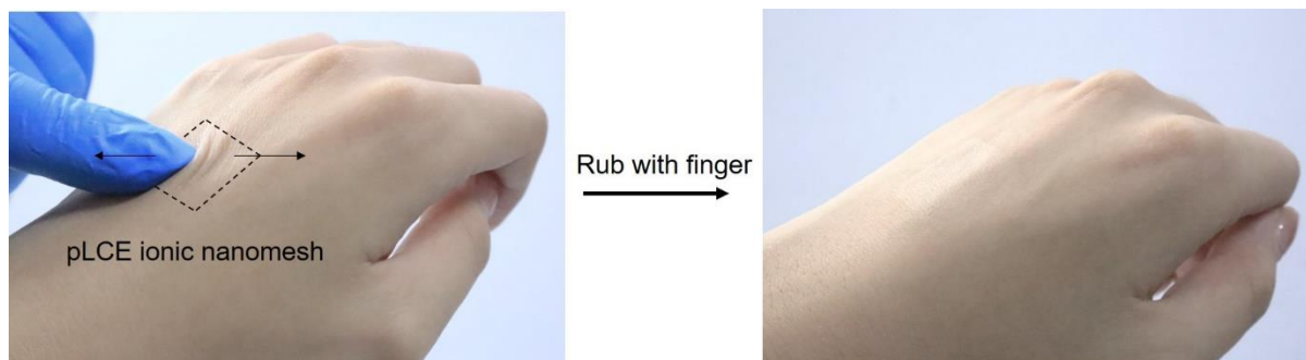
Supplementary Fig. 21. Scratch resistance of pLCE ionic nanomesh adhered on hand skin.
