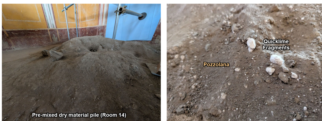
Supplementary Figure 4. Premixed pile of dry pozzolana and quicklime from Room 14 (left), and a higher magnified view (right) clearly showing the individual quicklime fragments.
