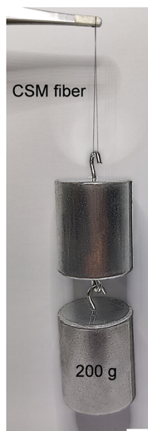
Supplementary Figure 26. Photograph exhibiting a folded CSM fiber lifting the weight of 400 g. Scale bar, 1 cm.
