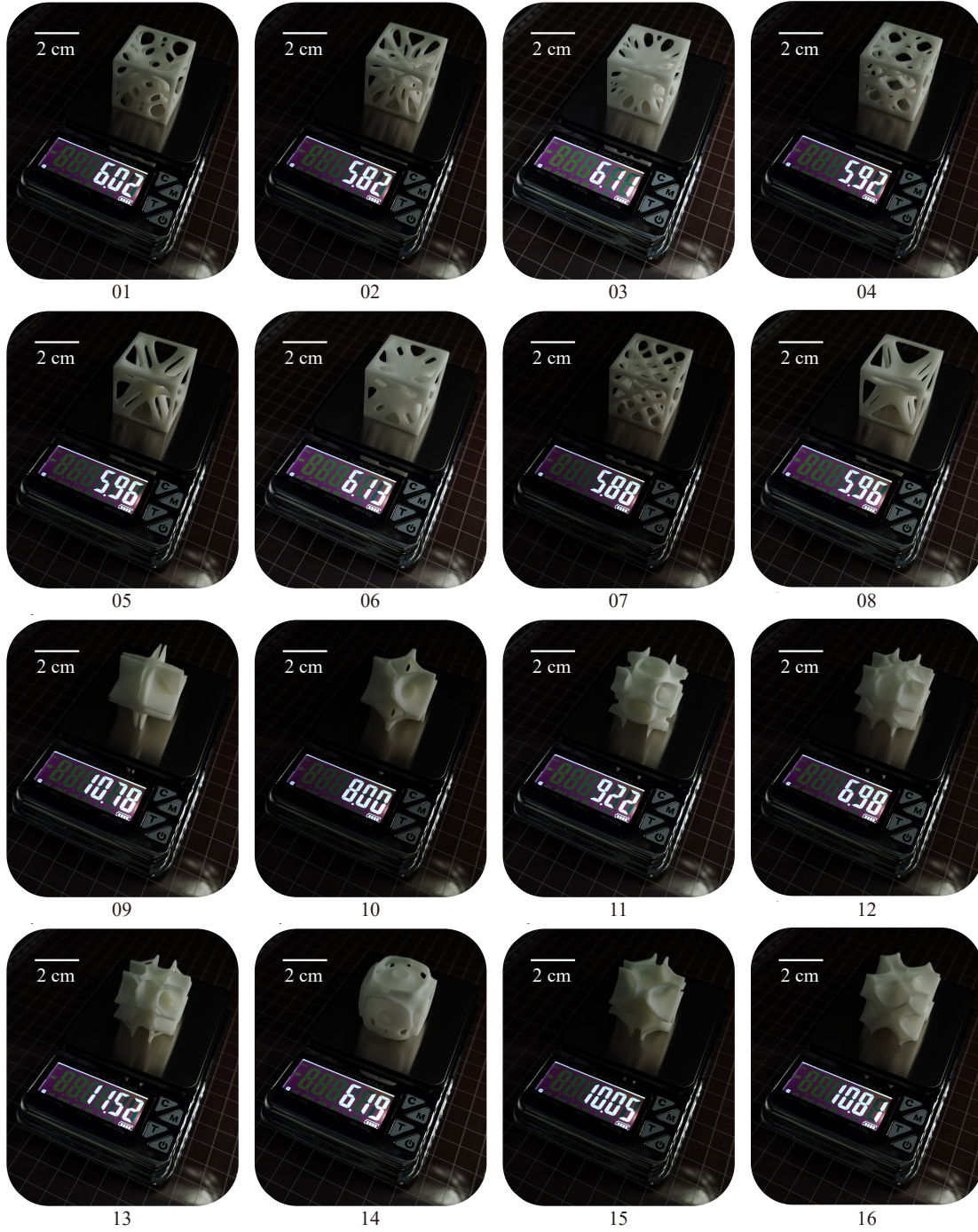
Figure S17: Measured mass of the 16 3D-printed photopolymer resin samples. 01-08: bicontinuous open-cell microstructures. 09-16: randomly selectly microstructures.
