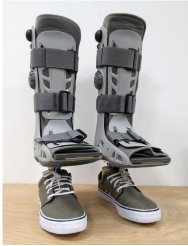
Supplementary Fig. 12 | Customised walking boots for preliminary testing of prosthetic feet with unimpaired subjects. Boots were customised by incorporating prosthetic adapters screwed to the bottom of their soles to enable attachment of the prosthetic feet. For plantar pressure mapping, sensorized insoles were placed into the shoes, under the prostheses.
