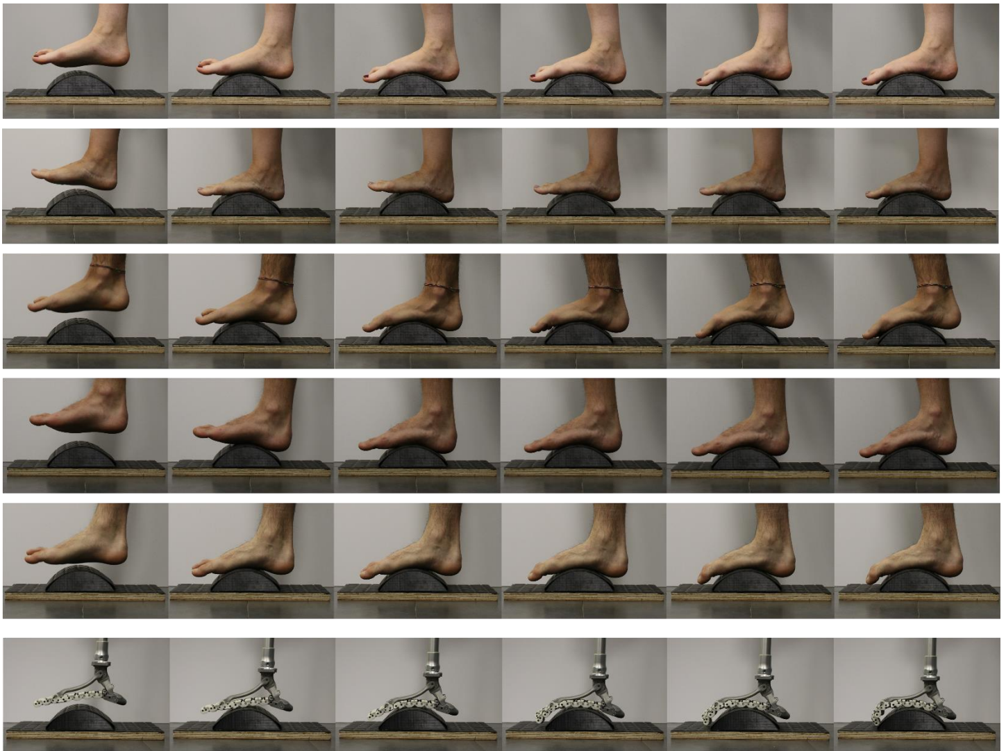
Supplementary Fig. 13 | Change in shape of the human feet (first five rows) and the SoftFoot Pro (bottom row) on an arch-shaped obstacle.
