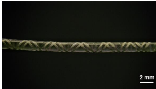
Supplementary Fig. 20. Optical image of a fiber (diameter, 1.5 mm) with two layers of EGaIn microcircuits.
