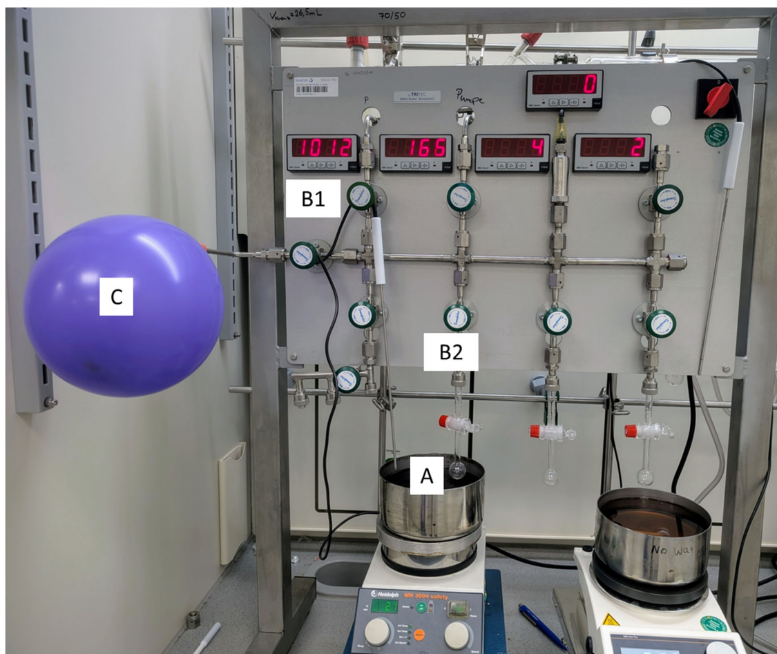
Figure S125: Deuterium manifold set up for HIE reaction.
