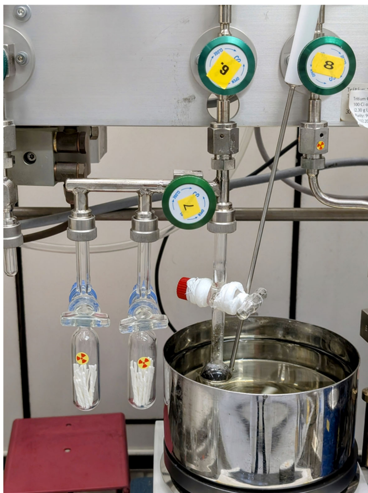
Figure S126: Tritium reaction set up.
