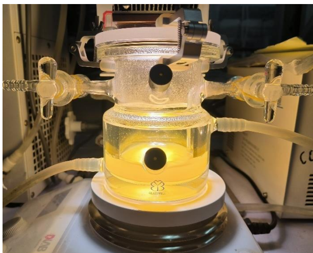
208 209 Supplementary Fig. 23 The photo of photocatalytic reactor. The photo of glass reactors for 210 photocatalytic CH 4 conversion evaluation. 211
