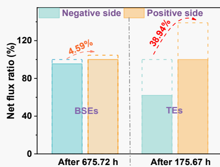
Fig. S23 Electrolyte net flux between the positive and negative sides in VRFBs with BSEs (P 1.91 M V^{3.55+} ; N 1.17 M V^{3.50+} ) and TEs (P 1.70 M V^{3.50+} ; N 1.70 M V^{3.50+} ) combining with N212 before and after cycling.
