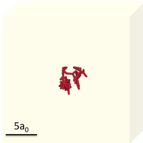
Supplementary Fig. 9. Trajectory of single vacancy diffusion in \text{Ni}_{80}\text{Mo}_{10}\text{W}_{10} at 1000 K for 5ns.
