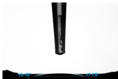
Figure S18. Pictures demonstrating the contact angle of hydrogels after swelling in distilled water.
