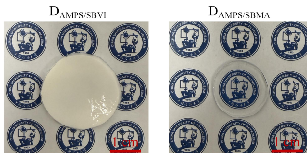
Figure S2. Morphological images of D_{\text{AMPS-SBVI}} and D_{\text{AMPS/SBMA}} hydrogels after swelling in water. D_{\text{AMPS/SBVI}} : The first network is AMPS and the second network is SBVI. D_{\text{AMPS/SBMA}} : The first network is AMPS and the second network is SBMA.
