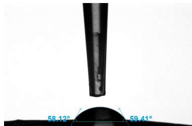
Figure S19. Pictures demonstrating the contact angle of hydrogels after swelling in brine.
