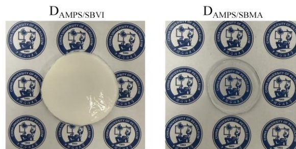
Figure R20. Morphological images of D_{\text{AMPS/SBVI}} and D_{\text{AMPS/SBMA}} hydrogels after swelling in water. D_{\text{AMPS/SBVI}} : The first network is AMPS and the second network is SBVI. D_{\text{AMPS/SBMA}} : The first network is AMPS and the second network is SBMA.
