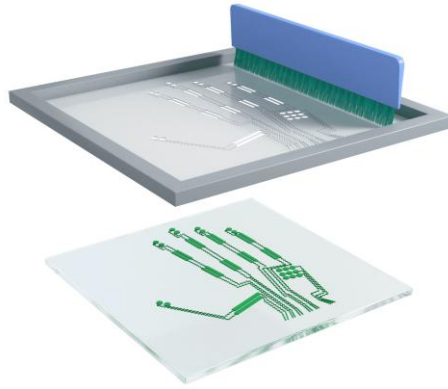
Supplementary Fig. 21. Schematic diagram of silver electrode screen printing. The electrodes were fabricated by screen printing silver paste through a 200-mesh screen onto a polyester fabric mesh coated with a photosensitive adhesive. This mesh was subsequently attached to a flexible TPU substrate 100 \mu\text{m} thick.
