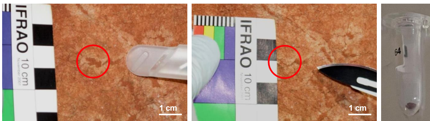
Fig. S2.4. Pigment sample SP.C.6764: cave wall before sampling (left); after sampling (middle); sample in tube (right).
