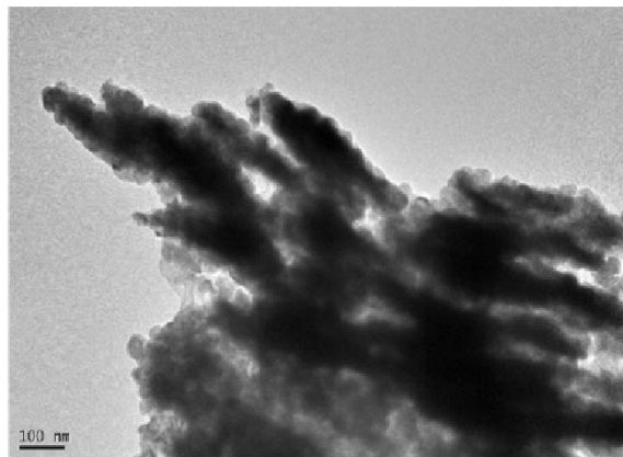
Supplementary Figure 14. HRTEM images of TCo-CuO NS catalysts after CO 2 RR.
