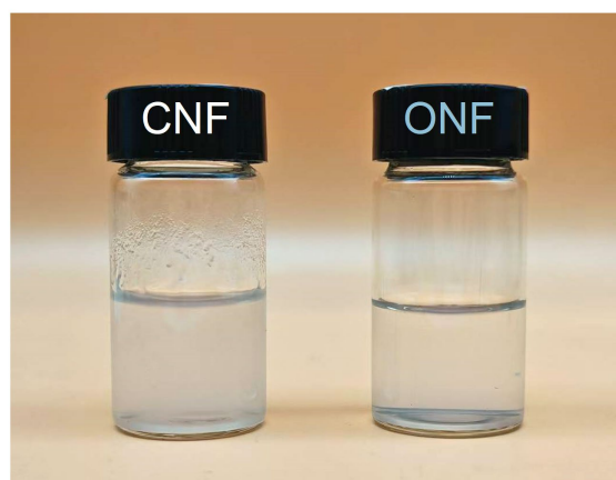
Supplementary Fig. 9. Optical photographs of CNF dispersion and ONF dispersion after three months of static storage at room temperature.
