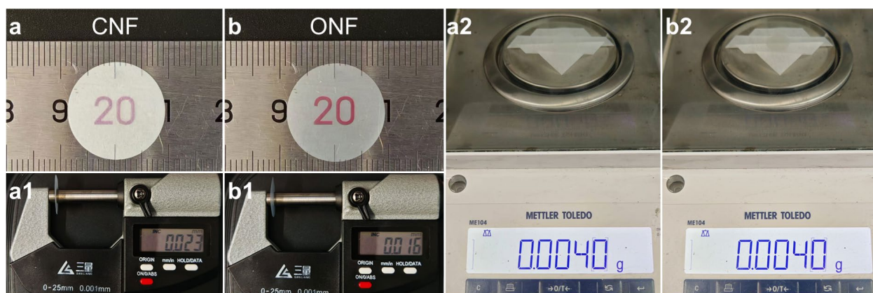
Supplementary Fig. 12. Thickness and mass comparison of a , a1 , a2 , CNF and b , b1 , b2 , ONF cellulose papers at equal surface area.
