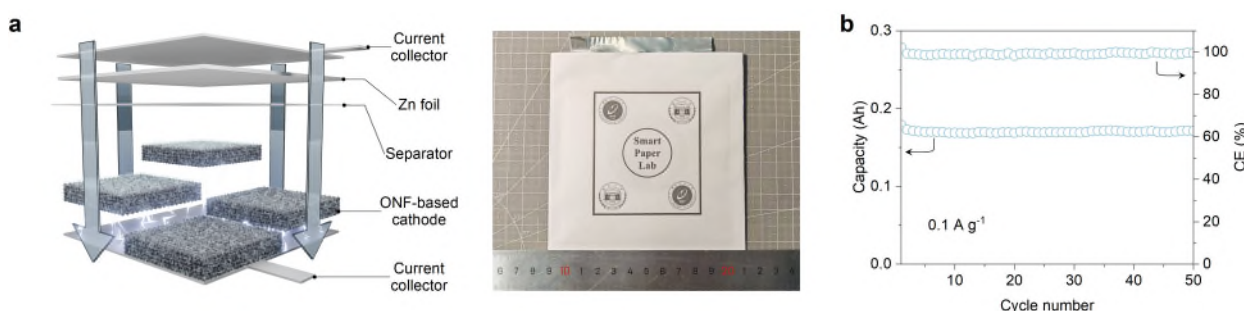
Supplementary Fig. 48. a, Schematic diagram, optical photograph, and corresponding b, electrochemical performance of the pouch cell with ONF-based high-loading iodine cathodes.
