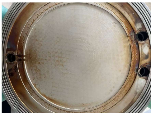
Fig. S67. Post-test photographs of the disassembled 1.0 kW ASWE showing the bipolar plate with three ports (electrolyte inlet/outlet, O 2 outlet, and H 2 outlet) after operation.
