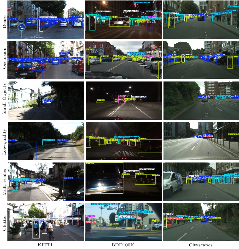
Supplementary Fig 3: Representative detection results of FAD on the KITTI, BDD100K and Cityscapes datasets. FAD in accurately detecting objects of traffic scenario, such as dense, occlusion, small objects, low-quality, multi-scale and clutter. Since the images we selected contain different scale objects, zooming in on the page gives a better visual effect. Images from the KITTI Vision Benchmark Suite are used with permission and made available under the CC BY-NC-SA 3.0 licence ( https://creativecommons.org/licenses/by-nc-sa/3.0/ ).
