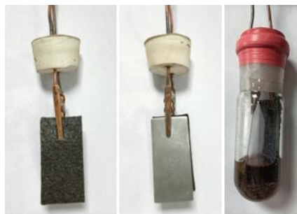
Fig S34. Electrolysis setup. A graphite felt and a stainless-steel plate (width: 1.8 cm; immersion depth: 0.56 cm) were used as the electrodes.
