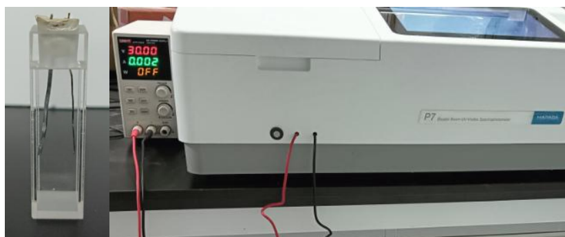
Fig S32. Setup of UV-vis spectroelectrochemistry. The electrochemical cell consisted of a zinc wire anode and a stainless-steel wire cathode.
