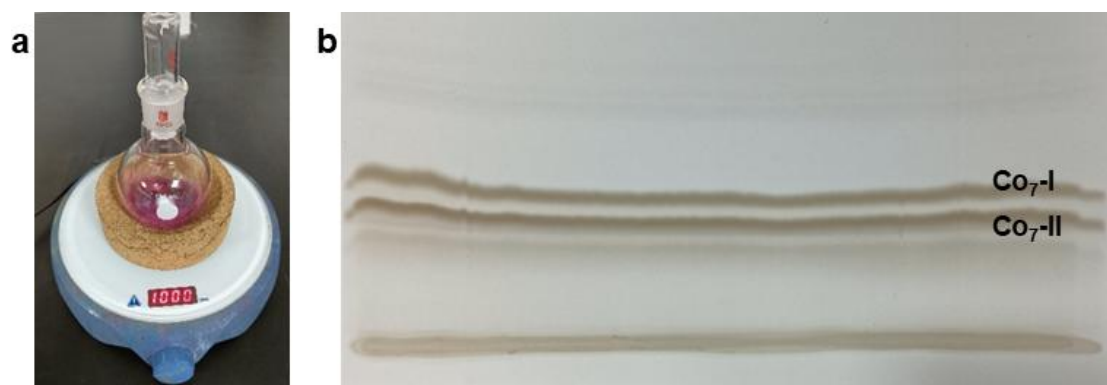
Fig S1. The synthesis of cobalt nanoclusters. (a) The reaction setup. (b) TLC picture of Co 7 -I and Co 7 -II with DCM/PE (1/1, v/v) as a developer.
