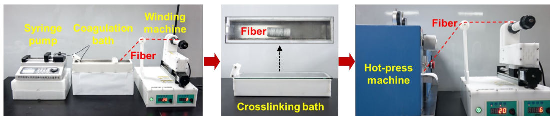
Supplementary Fig. 6. Optical images showing the apparatus for the mild fabrication of CS-MXene fibers, including wet-spinning, crosslinking, and hot-pressing processes.
