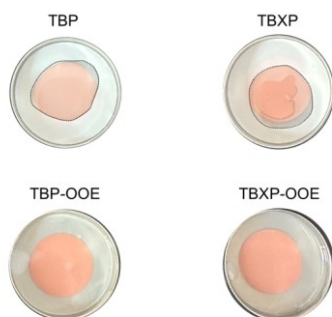
Supplementary Fig. 17. Wettability tests of the separator in different solvents.
