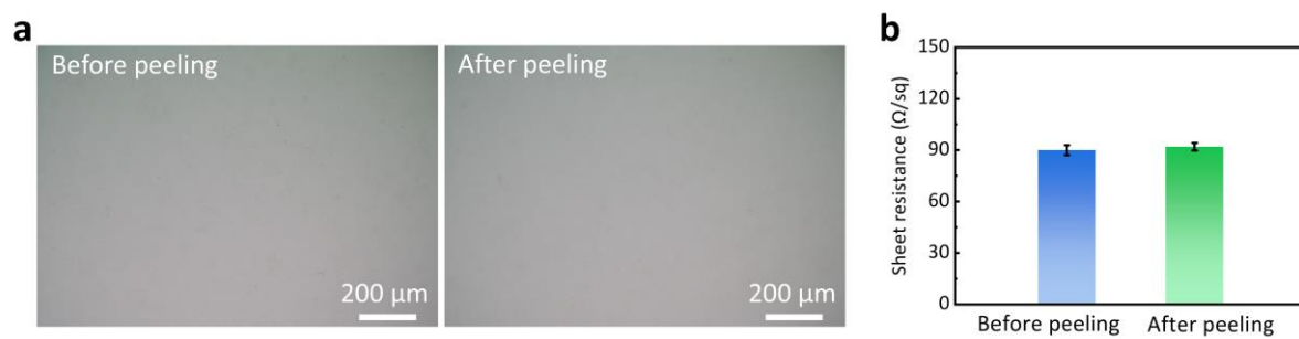
Supplementary Fig. S10 | Photographs of the embedded anode peeled from the OTS/Si substrate ( a ), and changes in the sheet resistance of the anode before and after peeling ( b ).
