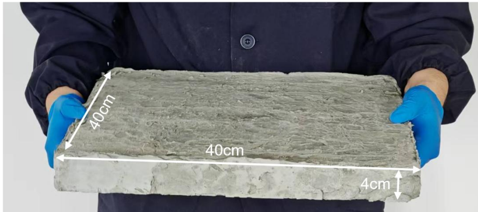
Supplementary Fig. 24. Fabrication of large-scale puff pastry architected cementitious material (PPAC) plate. Multiple PPAC blocks in the plastic stage were placed into a plastic mold measuring 40 cm × 40 cm × 4 cm. The contacting regions between adjacent PPAC blocks bonded together through slight vibration or compression, and after hardening, a large-size PPAC plate was successfully formed.
