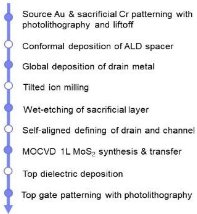
Supplementary Figure 2 Process flow for the fabrication of sub-5 nm channel arrays using a wet-etching process to remove the sacrificial oxide and metal layers. No electron-beam lithography or tape-assisted steps are required, ensuring CMOS compatibility.
