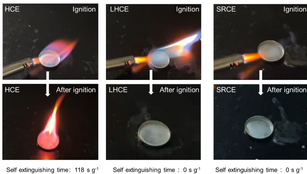
Supplementary Figure 40. Flammability test of different electrolytes. Optical images of during ignition and after ignition, alongside measured self-extinguishing times.
