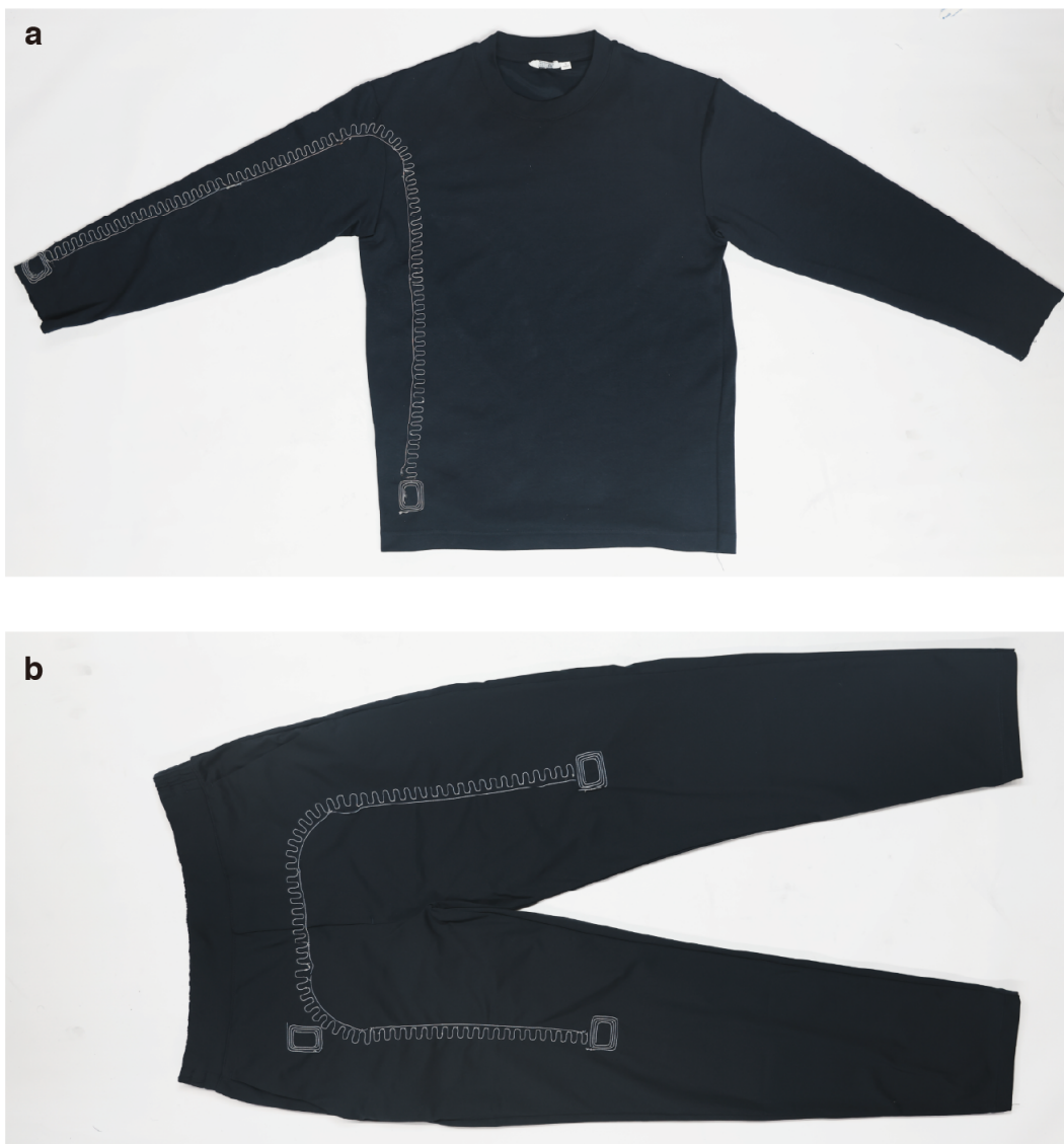
Supplementary Figure 41. The overall architecture diagram of the full-body WBSN. (a) Photograph of the upper garment WBSN. (b) Photograph of the lower garment WBSN.
