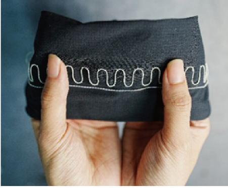
Supplementary Figure 8. Images of embroidered dual-mode metamaterial textile subjected to pristine and twisting. (a,b) The images are for demonstrating the stretchability and mechanical properties of the metamaterial textile.
