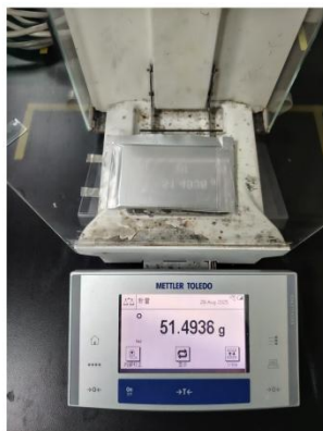
Supplementary Fig. 42 | Quality measurement of a 7.5-Ah lithium metal pouch cell with TFME electrolyte.
