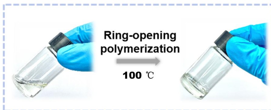
Figure S1. Crosslinking of BFDGE molecules occurred via ring opening polymerization of epoxide following a thermal treatment with IPDA as crosslinking initiator.
