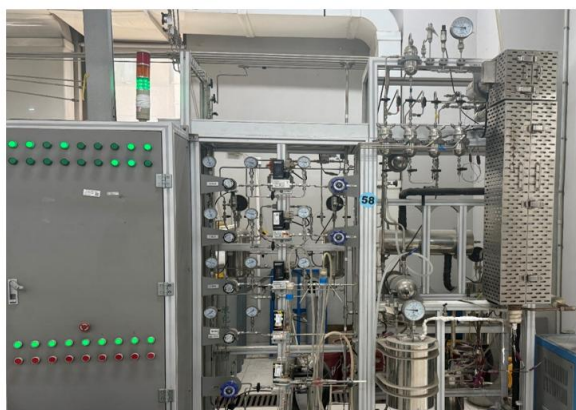
Supplementary Fig. 47 | (a) Photograph of the pilot-scale fixed-bed reactor apparatus. (b) Simplified schematic process flow diagram of the reaction system.
