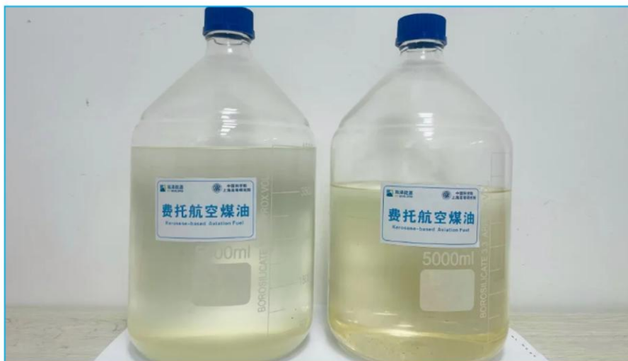
Supplementary Fig. 53 | Fischer–Tropsch jet fuel produced from the 1000 tonnes/year pilot unit.
