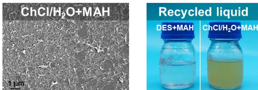
Supplementary Fig. S8. SEM images of CNF under the ChCl/H 2 O system and digital photos of its recovered solution.
