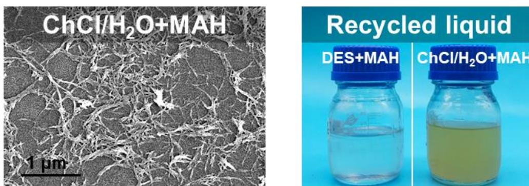
Supplementary Fig. S8. SEM images of CNF under the \text{ChCl}/\text{H}_2\text{O} system and digital photos of its recovered solution.
