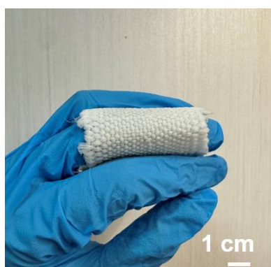
Figure S14. Optical photograph of the soft GP-BCAFs showing its woven-like structure and high flexibility. The sample is held with gloved fingers, and the scale bar represents 1 cm.
