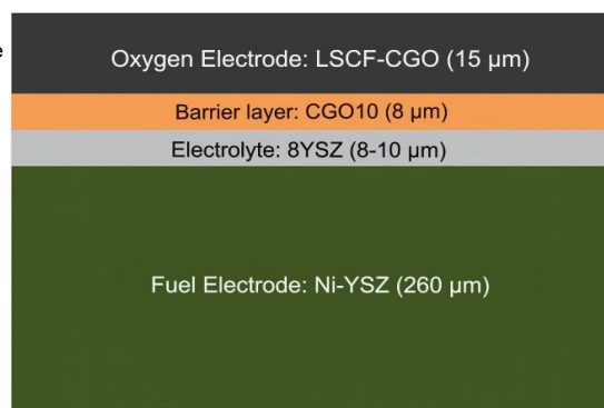
Fig. S1. Stack design and architecture of the single SOEC. a , Photograph of the assembled planar stack with metallic interconnects and compression hardware; b , Top view of a single repeating unit showing the sealing frame and flow field/rib structure; the dark central region corresponds to the electrochemically active area. c , Cross-sectional SEM of one cell highlighting, from top to bottom, the LSCF–GCO oxygen electrode, a thin GGO10 barrier layer, a dense 8YSZ electrolyte (8–10 μm), and the Ni–YSZ FE (~260 μm). d , Schematic of the layer sequence used in this study.
