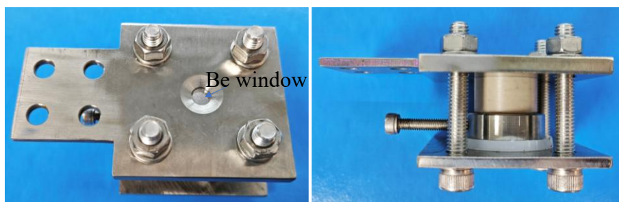
Supplementary Fig. 14. Digital image of the cell setup for operando I K-edge X-ray absorption spectroscopy measurement.
