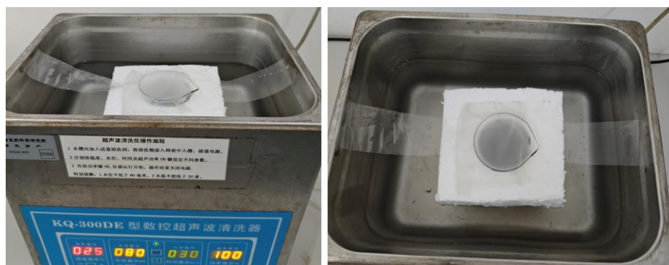
Figure S38. Experimental setup for microbial inactivation. The experimental setup used for microbial inactivation. 50 mg of PTFE particles with a particle size of 25 \mu\text{m} were added to 50 mL of DI water in a 150 mL beaker, followed by ultrasonication to obtain a dispersed suspension.
