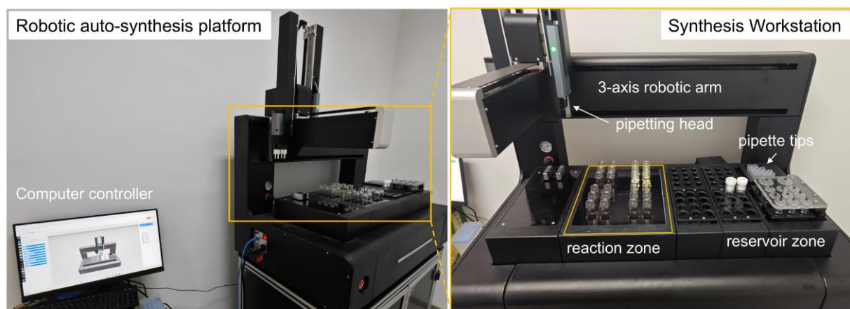
Supplementary Fig. 3 Photograph of the robotic auto-synthesis platform. The platform employs a computer-controlled robotic arm to aspirate precursors and synthesize PNCs in the reaction zone. This system enables high-throughput synthesis across a range of precursor ratios, thereby accelerating the optimization and screening of PNCs.
