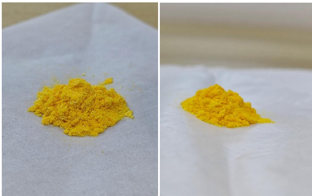
Figure S6. Digital photographs of \text{Cu}_{13}\text{H}_6 crystals. Crystal photographs were taken at room temperature.
