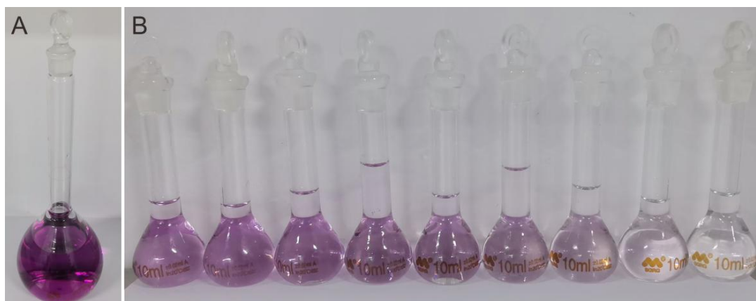
Figure S36. The photographs of Formazan standard solution (A), and the gradient dilution solution pictures (B). It shows the purple color of the solution.
