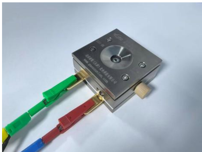
Supplementary Figure 64. Photographs of the customized battery device for in situ Raman measurement.
