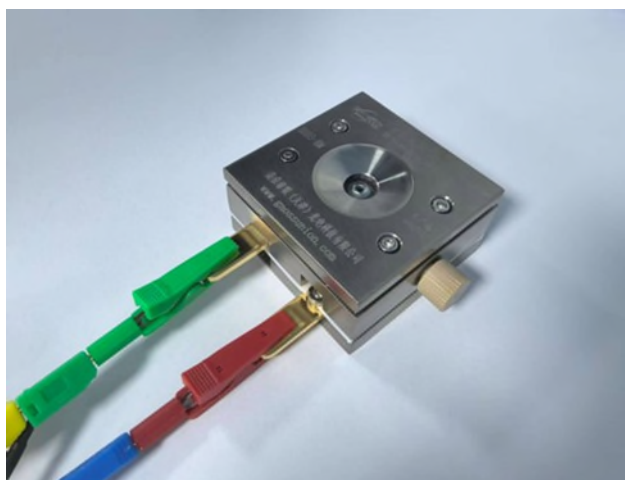
Figure R8. Photographs of the customized battery device for in-situ Raman measurement.
