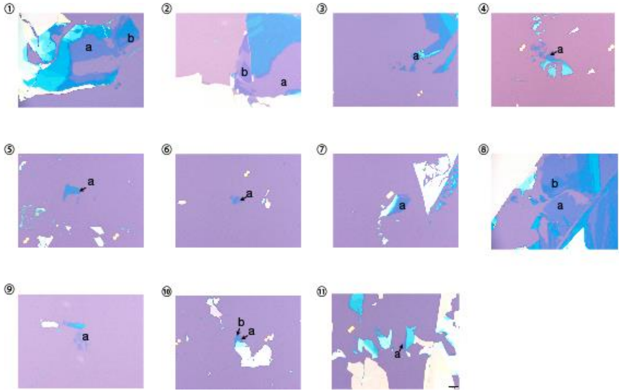
Supplementary Figure 1. 11 optical micro scope images of MoS 2 atomic layers for test data. The parts to be answered is shown as “a” or “b” in each image.
