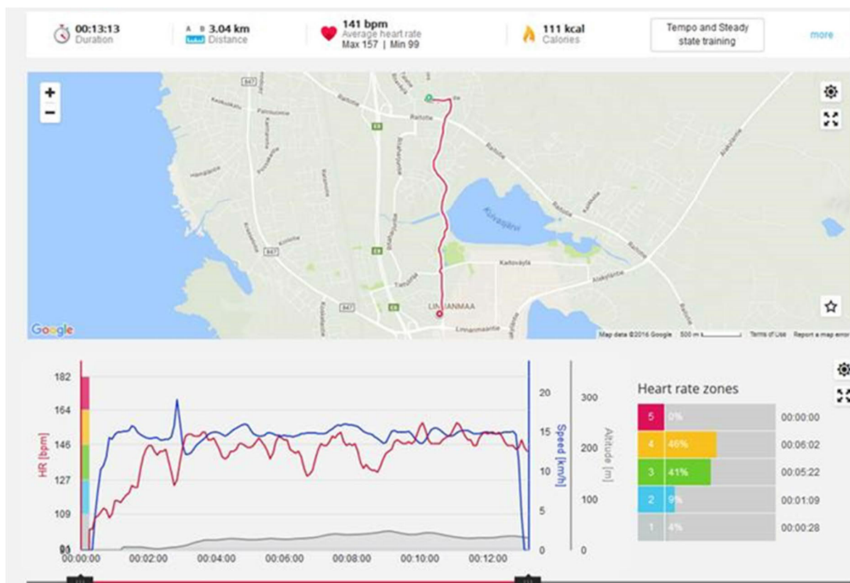
Figure S8. Results of suitability of the printed electrodes for commercially available heart-rate monitors. The plot demonstrates satisfactory data acquisition and response to the heart-rate changes over various conditions – valley in the hear-rate date plot at approximately 3 min is a result of cycling downhill.
