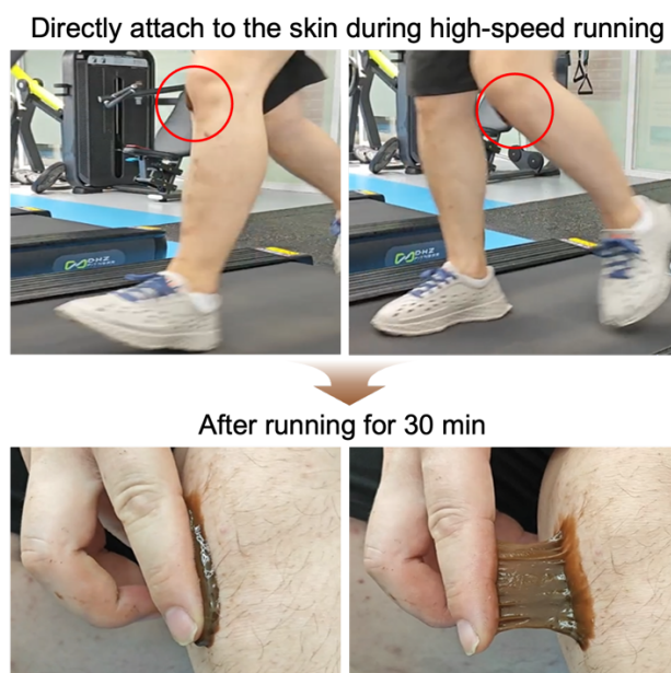
Supplementary Figure 15. The Ag@PDA-(CSPBA/CSGA) hydrogel attached firmly on skin during running.
