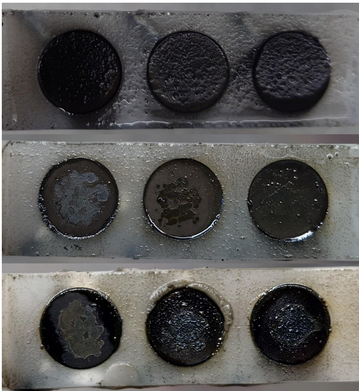
Supplementary Figure 1b. Photographs taken of the coupon rods taken from the biotic condition on Day 28, on dismantling the reactor, after exposure to anaerobic nutrient-enriched ASW media for 28 days.
