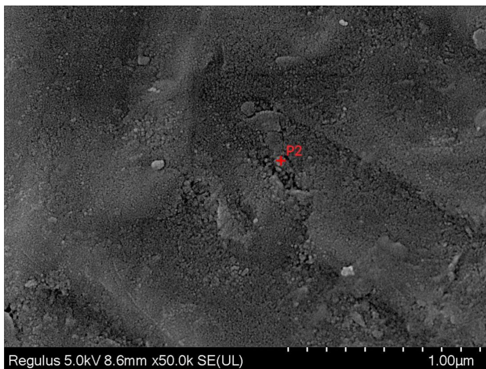
Figure S5. SEM image of the localized corroded region on glaze surface shows the nanoscale particles with varying packing densities. The chemical composition of P2 is listed in Table S1.
