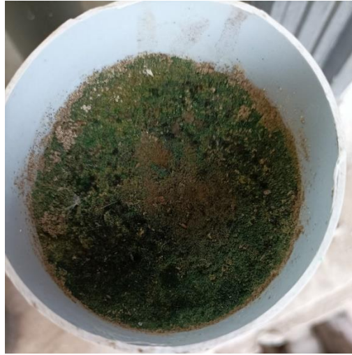
Supplementary Figure 1: Formation of Schmutzdecke layer on the top of the slow sand filter
