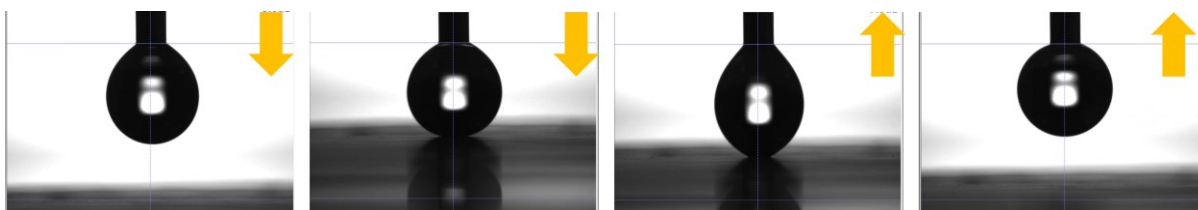
Fig. S6: Automatic dispenser attempting to deposit a 5 \mu L droplet on top of IPA-NIPS membrane. Yellow arrows indicate direction of needle/droplet movement.
