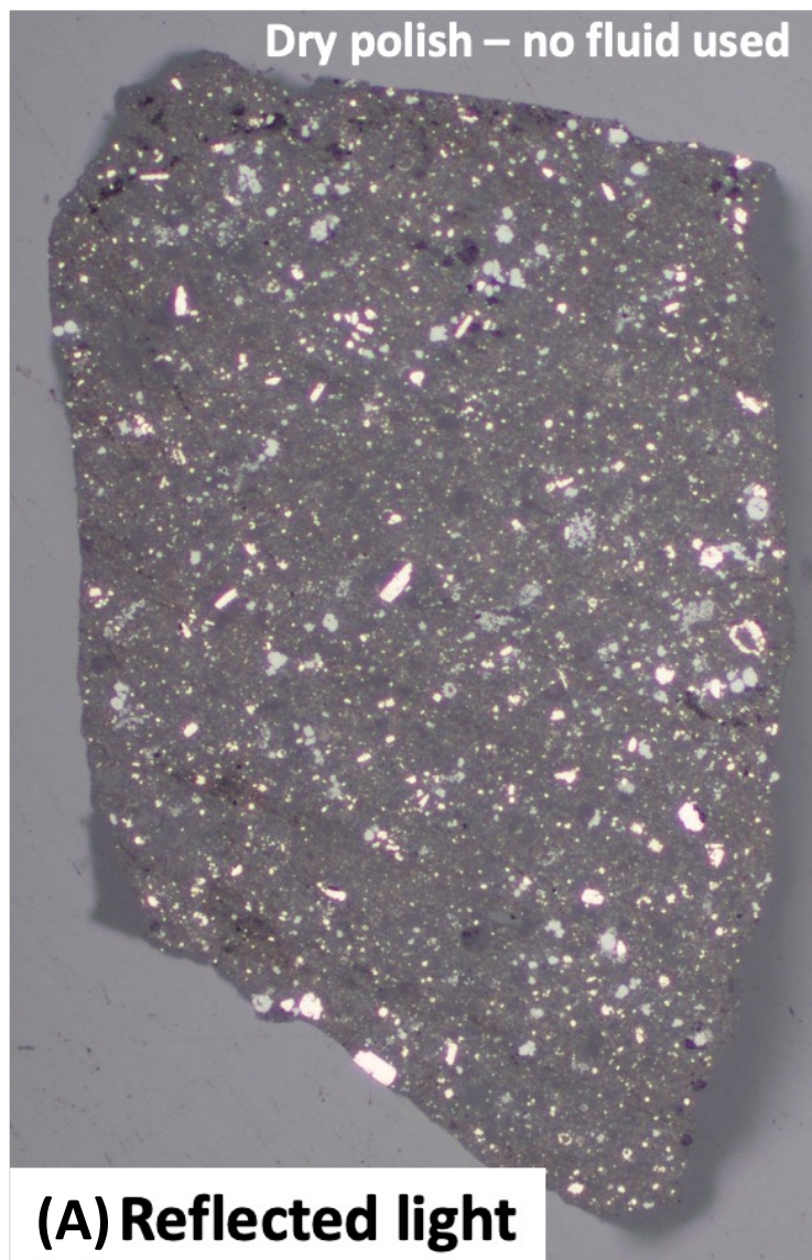
Supplementary Fig. 1. (A) reflected light and (B) back scattered electron images of Ryugu C0068.
