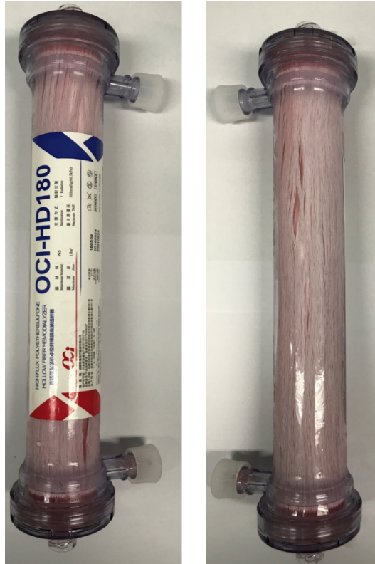
Supplementary Figure 32. Digital photos of the haemodialyzer (OCI-HD180) after blood purification. No obvious blood clot was observed in the haemodialyzer.
